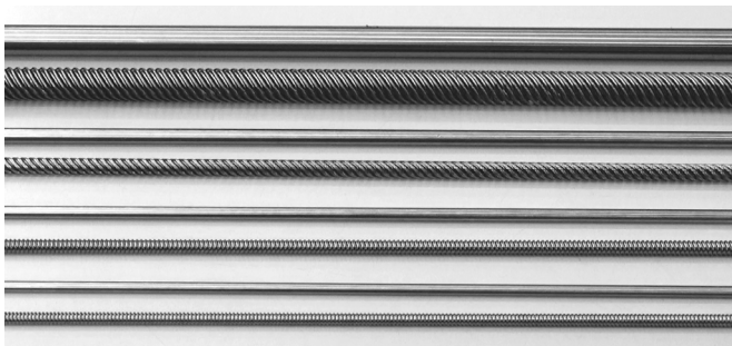
Fig. 3: Ball screw before and after rolling
